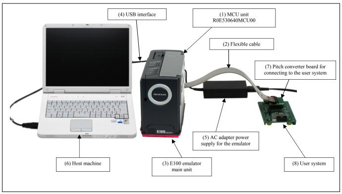
Figure 1.1 System configuration
